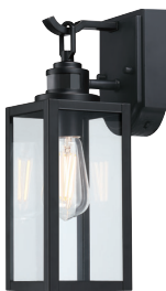
61226 Victoria Wall Fixture Matte Black Finish Clear Glass Height: 15.00" Width: 5.00" Extends: 7.25" Height from Center of Outlet Box: 3.35" Back Plate: H: 6.69" W: 4.72" Use (1) Medium (E26) Base Lamp, 60W Maximum
