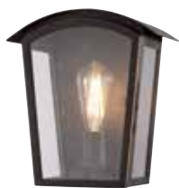
65802 French Quarter Wall Fixture Oil Rubbed Bronze Finish with Highlights Clear Seeded Glass Height: 10.75" Width: 10.00" Extends: 5.75" Height from Center of Outlet Box: 5.50" Back Plate: H: 8.66" W: 5.11" Use (1) Medium (E26) Base Lamp, 60W Maximum
