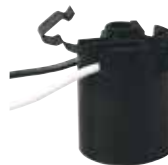
*22217 1 ½" Snap-in Socket 9" Wire Leads Medium Base Fits ¾" x ¼" Hole 18 Gauge 105° Leads 660 Watts Max., 250 Volts Height - 1½"
