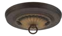
70050 Traditional Canopy Kit with Center Hole Oil Rubbed Bronze Finish 5 1/4" Diameter, 7/16" Center Hole, 50 lb. Load Rating Includes: 1 Canopy, 1 Crossbar, 4 Mounting Screws, 1 Lock Washer, 1 Locknut, 1 Screw Collar Loop, 2 Cap Nuts
