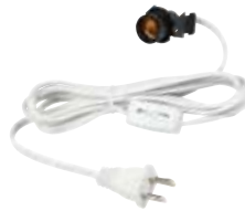
70108 - White 6' Cord Set with Snap-In Pigtail Candelabra Base Socket and Cord Switch No. 18-2, SPT-1, 105" Wire 75 Watts, 125 Volts Snap-In Spring Fits 1" Hole Switch is 12" from Socket
