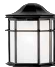
66898 Wall Fixture Textured Black Finish White Acrylic Lens Height: 10.00" Width: 7.75" Extends: 4.25" Height from Center of Outlet Box: 4.25" Back Plate: H: 9.38" W: 7.00" Use (1) Medium (E26) Base Lamp, 60 Watt Maximum
