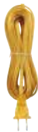
70103 15' Cord Set Gold Polarized Plug 18-2 SPT-2, 105" Wire Free ends are Split, Stripped and Tipped
