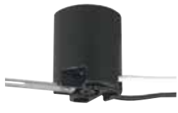
*22215 1 ½" Socket 6" Wire Leads and Straight Bracket Medium Base 18 Gauge, 105° Leads Bracket Extends 1½" Measured Center to Center 660 Watts Max., 250 Volts Height - 1½"
