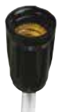
*22220 Pigtail Socket 24" Wire Leads Candelabra Base 18-2, SPT-1 105° Leads 75 Watts Max. 125 Volts Height - 1¾"
