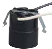
*22213 1 ½" Snap-in Socket 6" Wire Leads Medium Base Fits 1¼" Hole 18 Gauge 105° Leads 660 Watts Max., 250 Volts Height - 1½"
