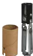
*22127 Adjustable Keyless Sockets Candelabra Base Threaded ½-IP Hickey 75 Watts Max., 125 Volts Height Adjustable from 3¼" - 4¾"
